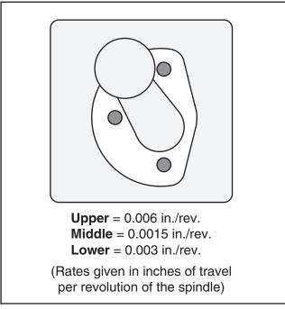
**Figure 38.** Positions of auto-downfeed rate selector.
